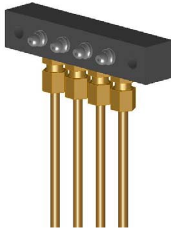
Fig. 37 Header Block with Grease Lines Connected to it.
